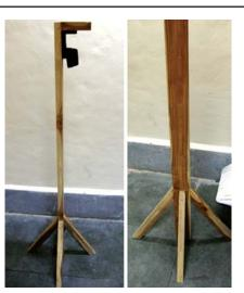
Fig. 10: To the left, note the simple wooden stand constructed to mount a CCTV camera (the black camera frame is seen) which will serve as the 'side' camera. To the right, note the base of the wooden stand that makes it extremely stable. The camera frame is at an approximate height of five feet
